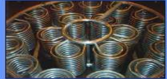
oil-steam heat exchanger
